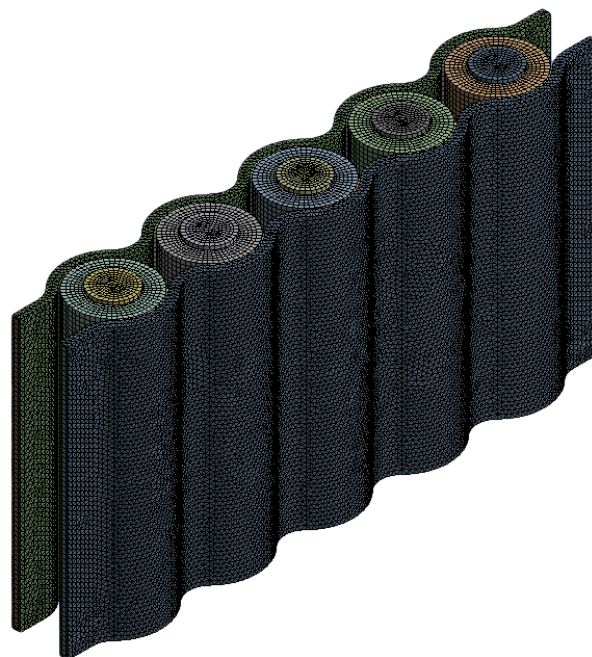
Figure 3. Meshing model for pack of lithium-ion battery.
