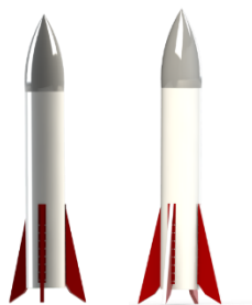
Figure 5. Three-fins rocket and four-fins rocket
